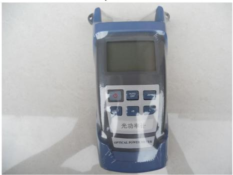
HYTT-OPM-RY3200B Handheld optical power meter is a compact and an easy-to-use testing instrument for optical fiber networks, which can be used for absolute optical power measurements as well as for relative loss measurements in optical fibers.
