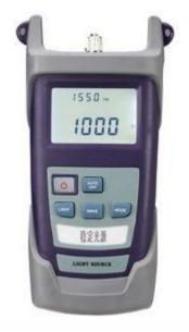
HYTT-RY-OLS-LS300 optical light source can provide 1 to 4 output wavelengths to meet specific requirements, including the 650nm red source and the 1310/1550nm wavelengths for single mode fiber or the 850/1300nm wavelengths for multimode fiber, as well as other wavelengths according to customer needs. Together with the HYTT-RY-PM-PM300 optical power meter, it is a perfect solution for the fiber optic network characterization.
